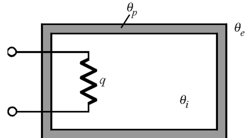
$$C_i \dot{\theta}_i(t) = k_{ip}(\theta_p(t) - \theta_i(t)) + q(t)$$
